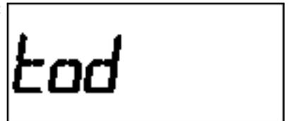
After "tod" is displayed, "12:00 PM" will display (or the current set time if already programmed) and the minutes will flash. The minutes are adjusted with the "+" or "-" key until the correct value is displayed.
