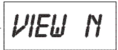
If "Y" is chosen, then pressing the "STATUS" key will display the value for salt dosage; repeated presses of the status key will display cycle times, batch capacity, and total capacity.
