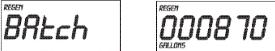
**Additional Features** - The Culligan Platinum Series Softener electronics are packed with features that expand the water softening experience. The statistics button allows you to view four separate gages: Capacity Remaining, Water Used Today, Average Water Usage, and Current Flow Rate. To view each item, press the statistics button, to step to the next item, press the button again. These screens will time-out after 5 seconds if no button is pushed.
