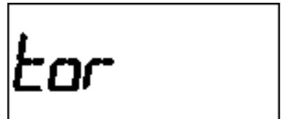
After "tor" is shown the display will then show the default of 2:00 AM (or the current programmed time of regeneration if already set). The time can be adjusted in 30 minute increments by pressing the "+" or "-" keys.
