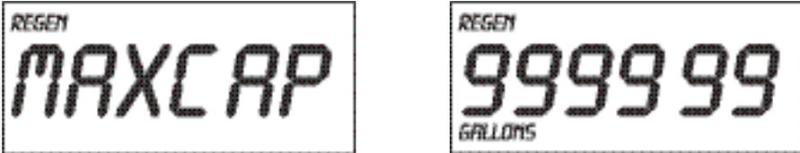
**Batch Set Point** - This setting is used to set the trip point for regeneration when in flow meter operation. It will only appear if a flow meter is connected, and 'dEFLtS' set to 'NO'. The programmed setting displays the actual set point to trigger regeneration. The display will show the "REGEN" icon and "BAtch" for two seconds and then display the "REGEN" and "GALLONS" icons and the setting numbers to adjust. Adjust the value with the "+" or "-" keys.
