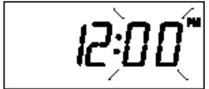
Pressing the "Status" key will move to the next programming step. Pressing "Regen" will move back to the minutes adjust.
