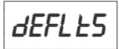
If 'YES' is chosen, then pressing the "STATUS" key will let the control automatically lookup, calculate, and save the values for salt dosage, cycle times, batch capacity, and total capacity, and proceed to the next item in the programming menu.
