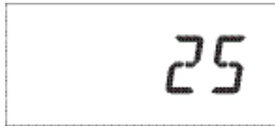
6. **Iron Setting (flow meter only)** - This setting is used to set the iron level (PPM) of the influent water supply. The display will show "Iron" in the left most digits and the iron default setting (or the previously programmed value) in the far right digit. The display will only appear if a flow meter is connected to the circuit board and the control is set to Gold, Platinum or Europe (softener only). Adjust the value with the "+" or "-" keys.
